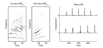
Figure 9: NMD analysis of the data in figure 8. The two words have been discovered as the objects described in the columns of the  $\mathbf{W}_t$  matrices. There respective location in time is denoted by spikes in the rows of  $\mathbf{H}$ .
