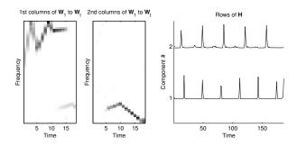
Figure 7: NMD analysis of the data in figure 5. Note how the spectral evolution character of the two objects is now captured by the structure of the  $\mathbf{W}_t$  matrices.
