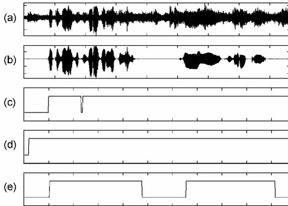
**Figure 4:** Comparison of VAD results for a speech signal in the presence of subway noise when the SNR changes temporally from 5 to 0 dB. The SNR of the first half is 5 dB, and that of the latter half is 0 dB. (a) Speech waveform mixed with subway noise. (b) Speech signal included in (a). (c) VAD result for (a) obtained with a statistical VAD method [6]. (d) VAD result for (a) obtained with ETSI AFE VAD [16]. (e) VAD result for (a) obtained with the proposed VAD method.
