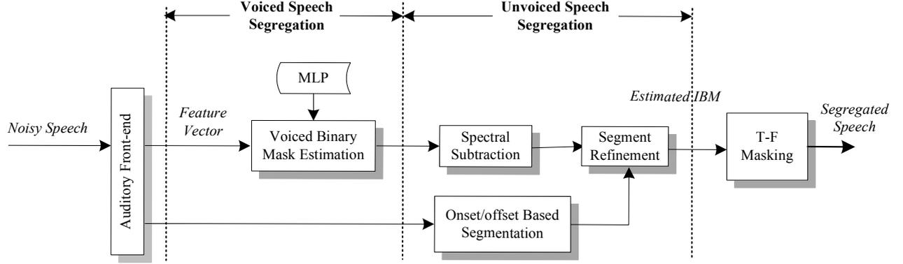
Figure 1: Schematic diagram of the proposed two-stage CASA system. In the voiced-segregation stage, the system uses a set of harmonic features to classify each T-F unit into target or interference. In the unvoiced-segregation stage, the system performs spectral subtraction on noise estimate from the first stage. In addition, onset/offset based segmentation is employed for segment refinement. The resulting time-frequency mask is then used to segregate the target speech.
